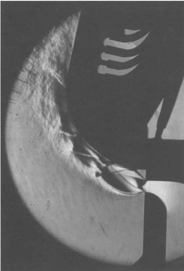
Figure 2 Planar model, spark schlieren near breakaway
